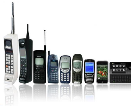
Fig.5: Example of technology trend shows increasing demand for smaller and compact design of electronic products that leads to higher heat dissipation and cooling capability requirement.
